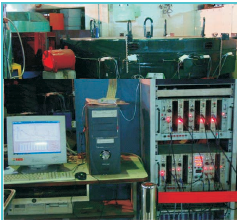
Upgraded Neutron Powder Diffractometer-I with new detector banks, radiation shielding and data acquisition system.
